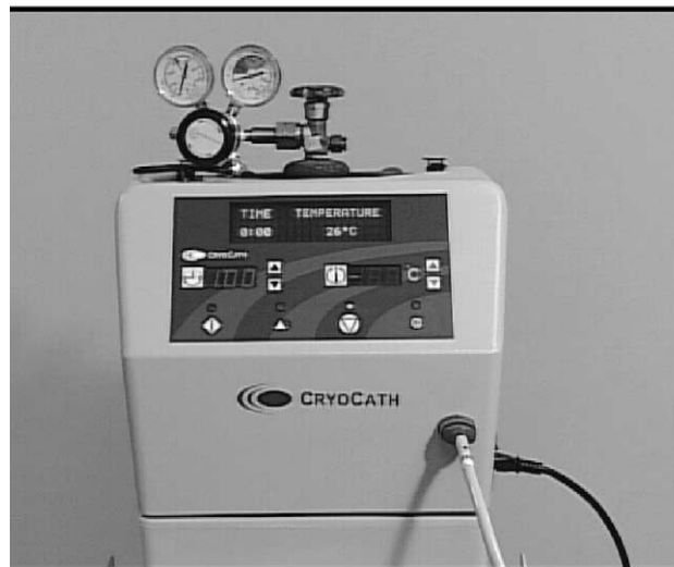
Fig 1. SurgiFrost CryoSurgical console. Cryoablation can be controlled by presetting temperature and duration of the system. Argon gas is used as a refrigerant.
